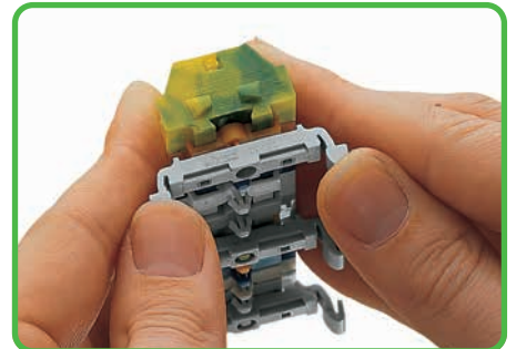
Terminal strip with snap-in mounting feet, connecting to 209-123 mounting adapter (The distance between mounting adapters should be 35 - 40 mm).
