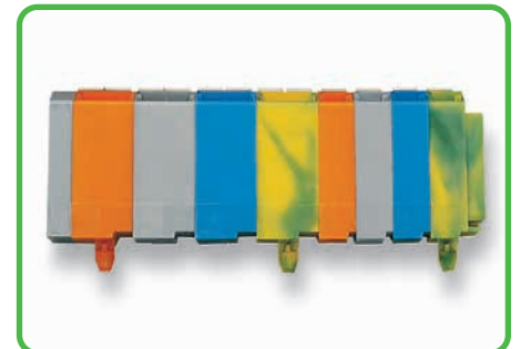
Terminal strip with snap-in mounting feet, for plate thickness 0.6 mm - 1.2 mm, fixing hole 3.5 mm Ø.
